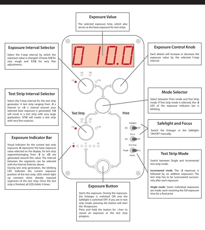
**Brightness Adjustment:** Switch the timer OFF. Press and hold the Exposure Button. Switch on the Timer (keep the button pressed!). You can now change the LED brightness by rotating the Exposure Control Knob. Release the Exposure Button to save the new brightness value.
